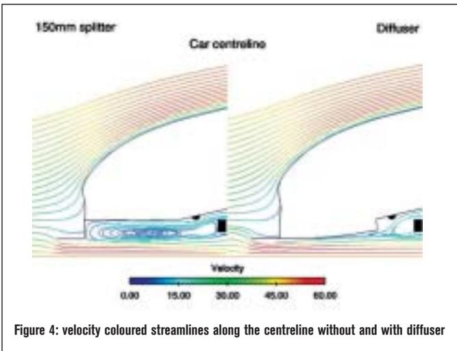
Figure 4: velocity coloured streamlines along the centreline without and with diffuser
