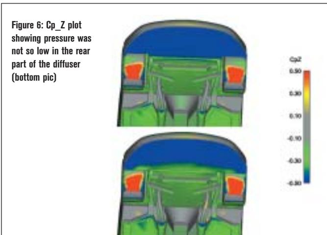
Figure 6:  $C_p_Z$  plot showing pressure was not so low in the rear part of the diffuser (bottom pic)
