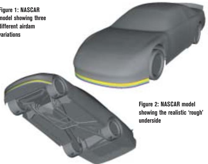
Figure 2: NASCAR model showing the realistic 'rough' underside
