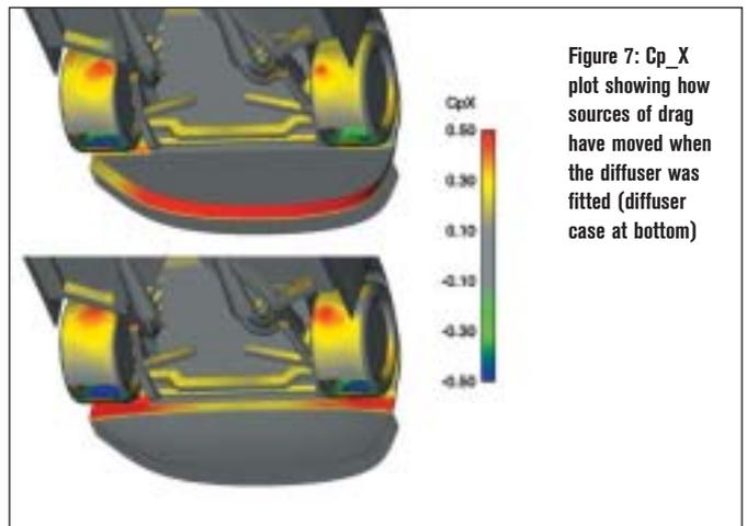
Figure 7:  $C_p_X$  plot showing how sources of drag have moved when the diffuser was fitted (diffuser case at bottom)
