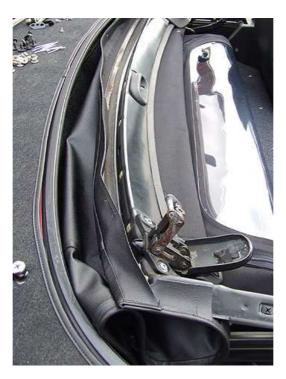
Install the header rail back in place using the screws removed earlier. Start with the centre screw to locate the header and then work outwards. The holes in the header rail should line up with corresponding holes in the front of the hood.
