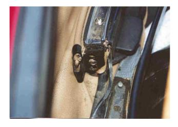
Next take the trim tool and remove the Rain Rail retainer stud from each side. To find these studs (the same as hold the carpet in place) look into the space close to the frame hinge with the top folded back and look towards the outside of the car. The stud is on the upper edge close to the front of the hinge cavity. The picture below should help you locate the studs.
