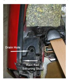
Once this is removed, use the drill to remove the two rivets exposed when removing the rear seal retainer on each side. Raise the hood and gently pry the rain rail from the back of the car away from the 13 captive bolts that pass through it. Take great care doing this as the rain rail is incredibly fragile and can be damaged easily when removing it.
