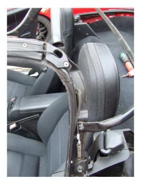
With the cables now in place, pull the hood material down and over the bottom of the B pillar as (there is a flap of material that "folds" over the bottom of the frame here with three holes in it) – it can help to have the hood frame tilted back slightly here to remove a little of the tension from the hood material.
