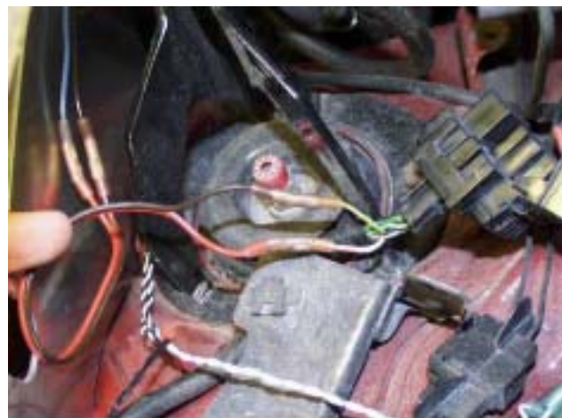
Wires from the boost control solenoid connected to the White/Red and Green/Yellow wires under the diagnostics connector.
