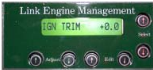
Press both the edit buttons to change the IGN TRIM screen to the CAS set up screen.
