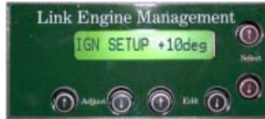
In this screen and only this screen, set the CAS to 10*BTDC with a timing light.
