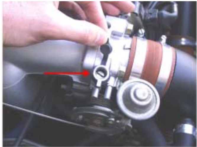
Idle screw on the side of the throttle body. 1.6L
