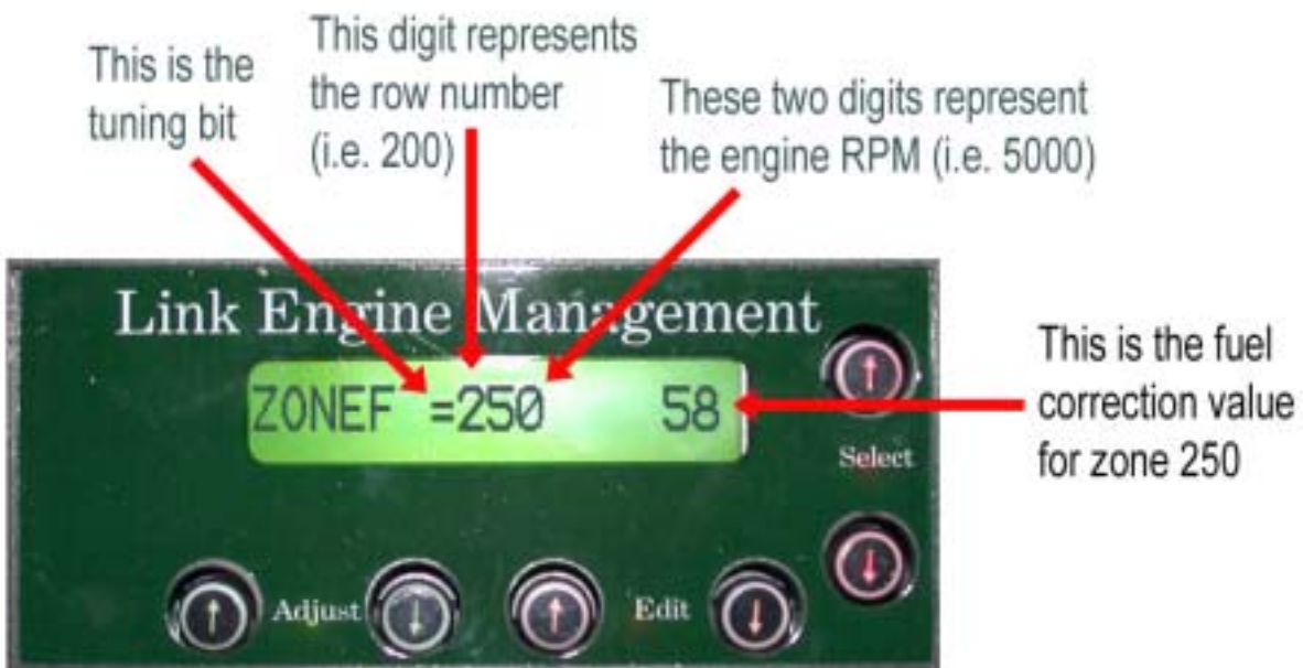
Link keypad in the ZONEF window for coarse fuel tuning
