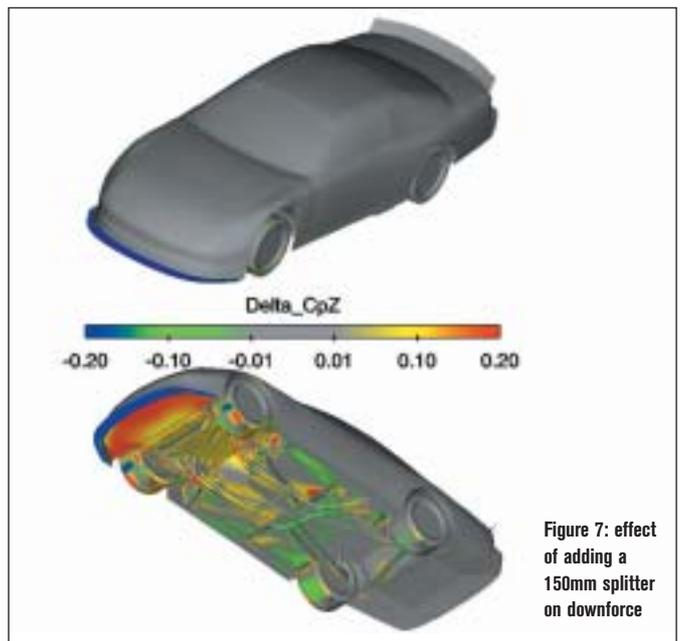
Figure 7: effect of adding a 150mm splitter on downforce
