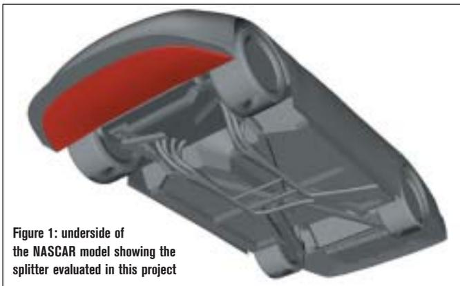
Figure 1: underside of the NASCAR model showing the splitter evaluated in this project
