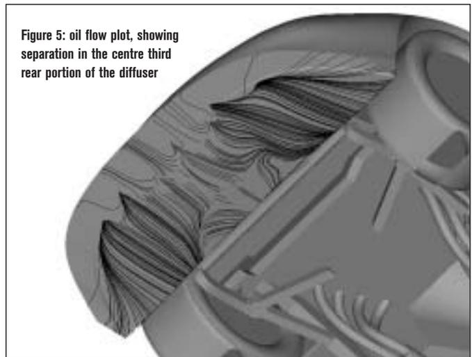
Figure 5: oil flow plot, showing separation in the centre third rear portion of the diffuser
