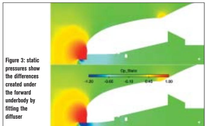
Figure 3: static pressures show the differences created under the forward underbody by fitting the diffuser
