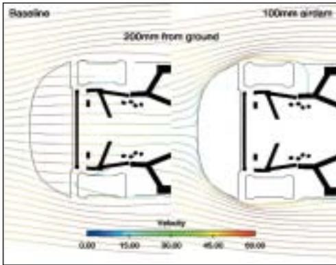
Figure 6: effect on downforce of adding a 100mm airdam
