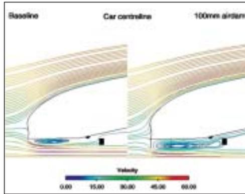
Figure 5: side view of streamlines at the car centreline for the no airdam and a 100mm airdam
