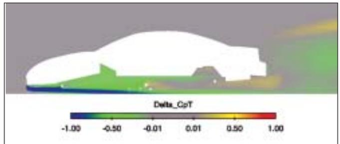
Figure 9: effect of adding a 100mm airdam on total pressure movement around the car
