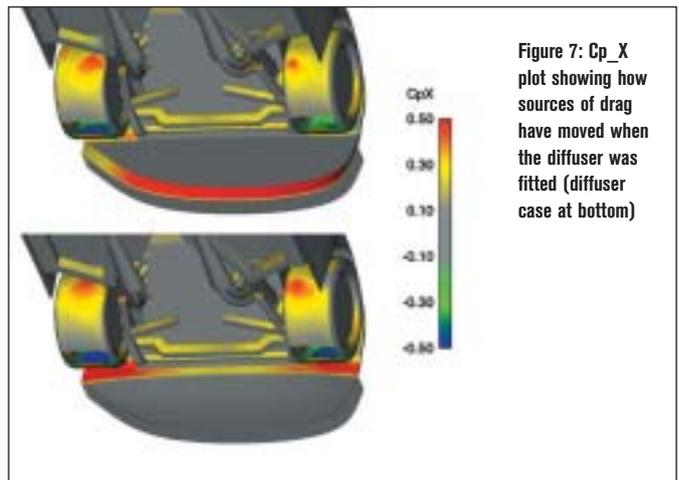
expansion the diffuser promotes increased flow under the splitter. This results in an increase in velocity under the splitter, which contributes to the decrease in static pressure there, in true Bernoulli fashion. There are also losses here resulting from the sharp leading edge of the splitter that cause a drop in total pressure and hence, a further drop in static pressure, though this is not evident in the diagrams here.
