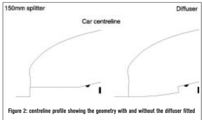
Figure 2: centreline profile showing the geometry with and without the diffuser fitted
