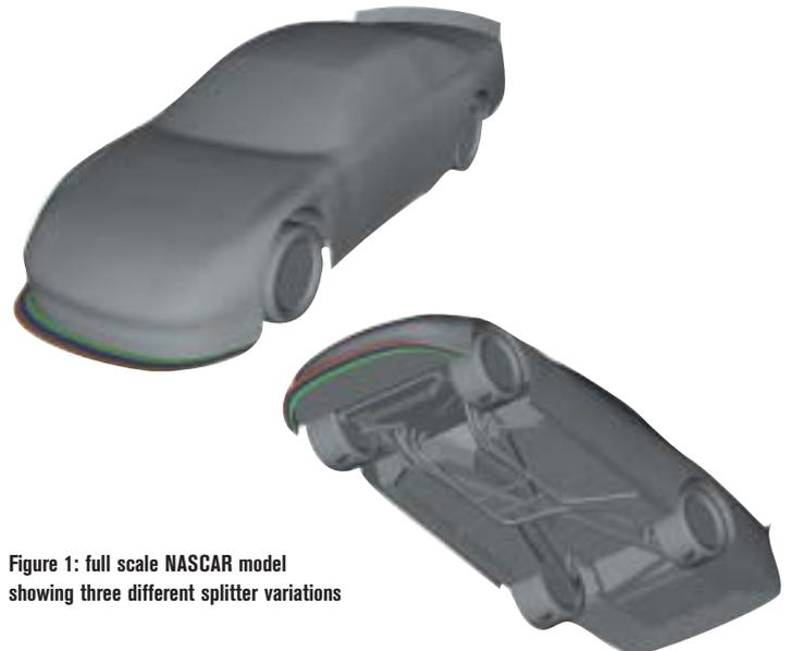
Figure 1: full scale NASCAR model showing three different splitter variations
