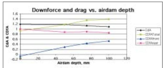
Figure 3: effect of airdam length on downforce at the front and rear, and overall drag
