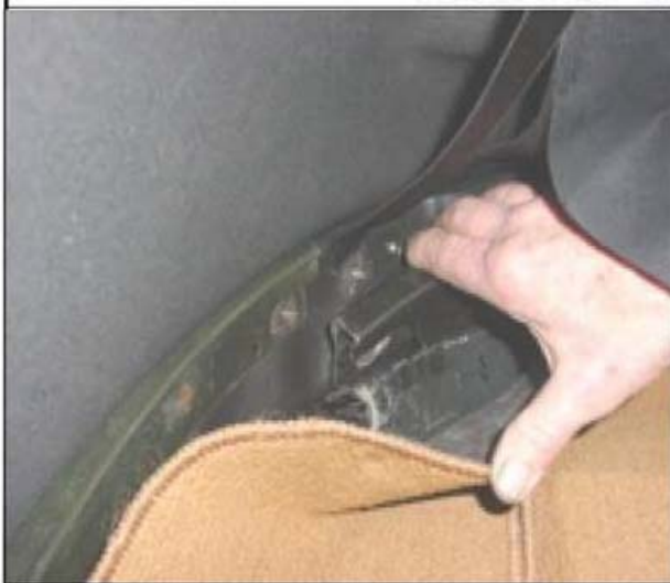
WEBBING STRAPS: Be sure to install the 2 webbing straps over the correct studs. See page 7 for correct stud locations.
