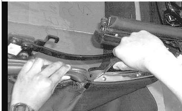
B PILLAR SEAL FASTENERS: Pull the 2 push type fasteners from lower B pillar.
