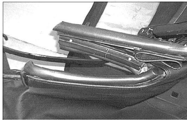
WEATHER SEALS: Remove the weather seals from their retainers.
