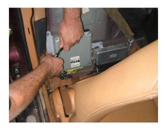
Remove the ECU, plug the OEM connectors into your new harness and attach the DB37 connector to your MS (be certain to screw in the connectors).
