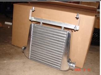
Place the intercooler upright and attach the upper mounting bracket with the provided bolts. The top and bottom mounting bolts can be found on the intercooler.
