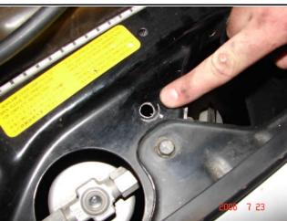
14.5 inches from the center of the first bolt and parallel to the radiator, drill another hole. For accuracy, drill a smaller hole first and then use a larger drill bit.
