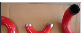
Next install the pipe coming off the turbo. The longer side attaches to the turbo. Use the 2.0 inch couplers and 2.0 inch tbolt clamp to mount this pipe.
