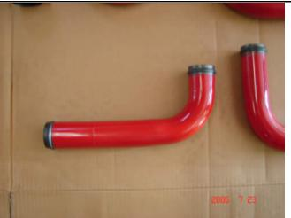
Next attach the lower L-shaped pipe to the pipe coming off the intercooler. The shorter side attached to the previous pipe. Use the 2.5-2.0 inch transition coupler for this connection.
