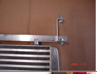
Remove the finishing bolt and washer and tighten the upper mounting bolt to the bracket on both sides.
