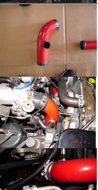
Attach the Throttle body pipe to the throttle body and attach it to the lower intercooler pipe. Use the provided 2.5 inch couplers and t-bolt clamps for each connection.
