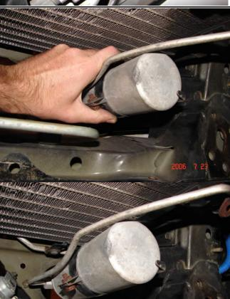
If you have AC, reach up and carefully squeeze your ac dryer lines. This will allow the mounting bracket room for installation
