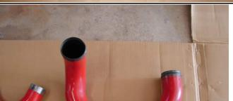
Start by attaching the bottom passenger side pipe to the intercooler. Use the provided 2.5 inch coupler and t-bolt clamps to attach to the intercooler. Tighten enough so the pipe stays in place, but do not completely tighten.
