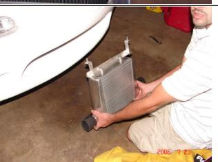
If you have an extra set of hands great. Otherwise you can mount this intercooler fairly easy. From underneath, carefully guide the intercooler into place and gently slide the upper bolts through the holes you just drilled. It's helpful to place the washers and finishing bolt near the holes beforehand so you can easily bolt the intercooler into place
