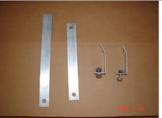
There are two different aluminum bars that fit each side. Bolt the labeled bar to the correct side of the car.
