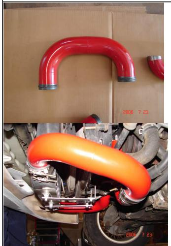
Attach the driver side bottom pipe. The shorter side attaches to the intercooler
