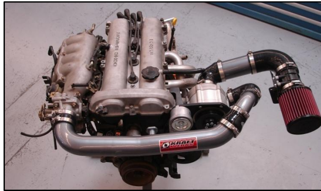
Figure 30: Crossover Tube Installed
