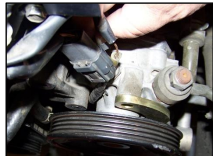
Figure 8: Re-route crank angle sensor wiring
