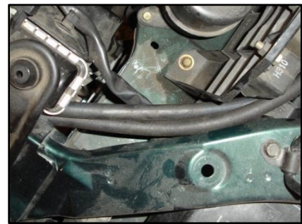
Figure 19: Driver's side oil hose routing
