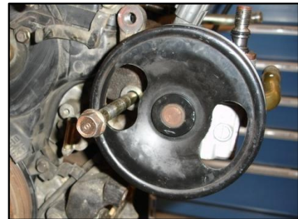
Figure 4: Remove power steering pivot bolt
