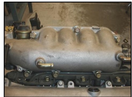
Figure 31: Remove intake manifold bolts
