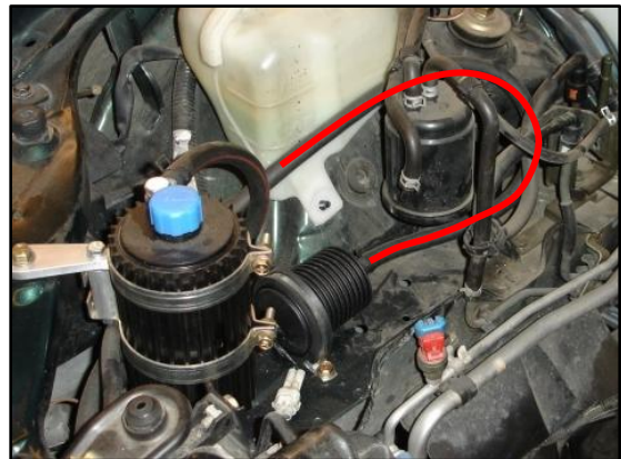
Figure 22: Loop in 89" oil hose
