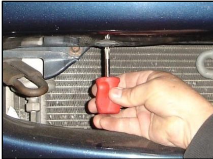
Figure 17: Plastic retainers in cowl
