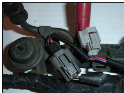
Figure 35: SuperCard harness properly plugged in
