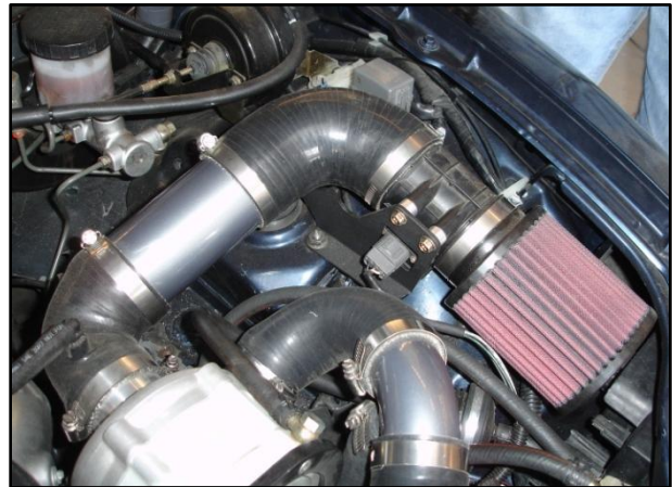
Figure 29: MAF Location and Hose Routing
