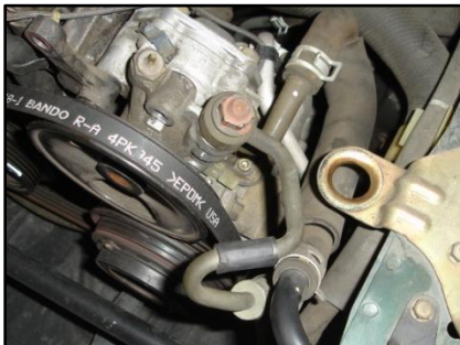
Figure 5: Rotate power steering hose for supercharger bracket clearance
