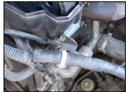
Figure 1: Upper wiring harness bracket
